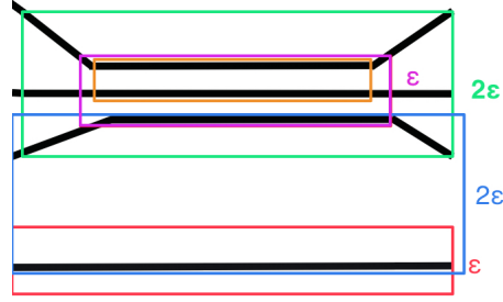
■ Figure 1 Bundles with different parameters: k=1 (red), k=2 (blue, orange), k=3 (pink, green). All bundles except the orange one are maximal. The green bundle is stable, the blue bundle is not.
