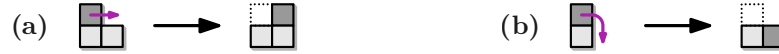
■ Figure 1 Moves admitted by the sliding cube model: (a) slide, (b) convex transition.
