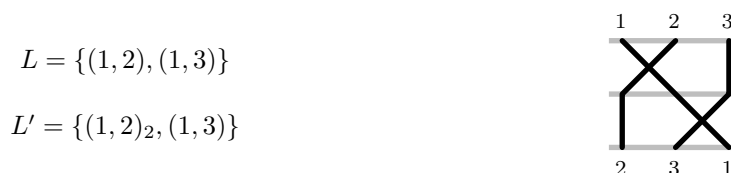
■ Figure 1 Lists L and L' for three wires (left). The list L is feasible (a tangle realizing L is to the right), whereas L' , which has two copies of the swap (1, 2) , is infeasible.
