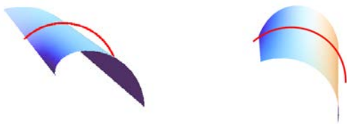
Figure 2: Sweep surfaces \mathbf{S}_1(s, t) and \mathbf{S}_2(s, t) , generated by the rational approximation to the RMF (left) and by the FSF (right).
