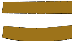
Figure 1: A simple test part produced by laser sintering that ends up with a slight U-shaped deformation.
